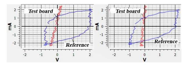
According to the form of this I - V characteristic, we can say that the tested board has a short to ground through a small resistance, probably this is the resistance of the burned out microcircuit itself, and on the standard we see the I - V characteristic of the pn junction + large capacitor chain.
