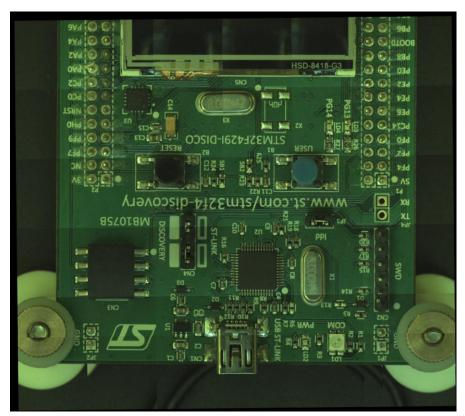
When connected to a PC, the board should be identified as ST-Link, but this did't happen, the board was recognized as an Unknown device. Also, when connected, the U1 microcircuit was heated. Based on this, it was assumed that the problem lies in the part of the ST-Link
