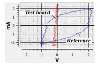
The difference between the I - V characteristic of the tested board and the reference one at the points marked in blue and red is most likely due to a problem in the U1 microcircuit. Therefore, we will try to determine what kind of microcircuit it is. To do this, you need to use the diagram or the list of components for the board.
