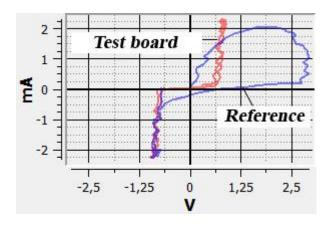
The resulting I - V characteristic indicates that there is an additional problem in the pn junction + capacitor circuit - there is no capacitance, which indicates a capacitor breakdown.
