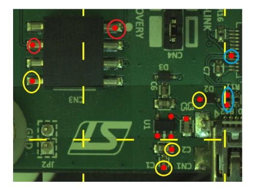
The points highlighted in yellow are connected to pin 3 of the U1 microcircuit as they have the same VAC.
