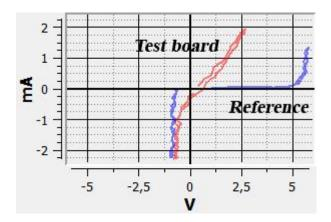
This current-voltage characteristic indicates that the output responsible for one of the USB lines (according to the datasheet on the microcircuit, this is the USB\_D- line) behaves incorrectly. This is the cause of the observed error when the device is identified as ST-Link, but with a communication error. Replacing this microcircuit and its firmware will eliminate the error and return the board to correct functioning.
